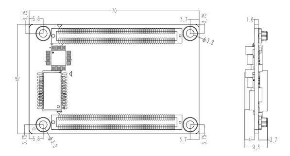
\* The board-to-board high-density connector has a combined height of 5.0mm and it is recommended to use a 5.0mm copper column.
