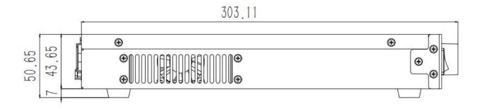
Unit: mm Unmarked linear and angular dimension tolerances comply with GB/T1804-M
