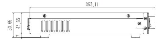
Unit: mm Unmarked linear and angular dimension tolerances comply with GB/T1804-M
