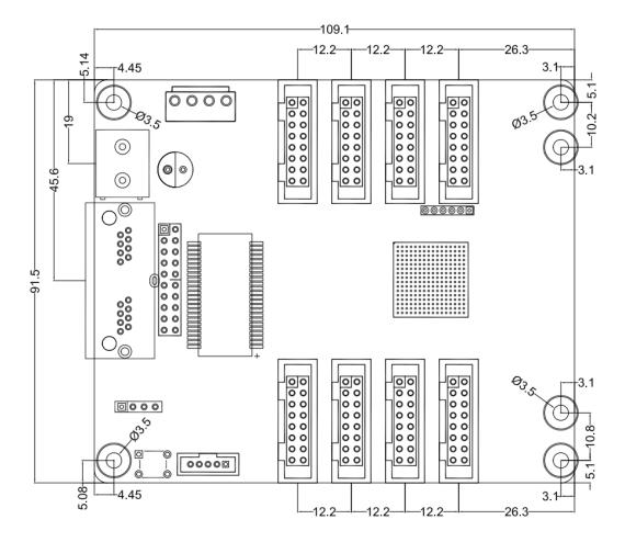
Unit: mm , tolerance  $\pm$  0.3mm
